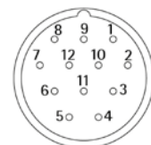
M23 12-pin cw connector
